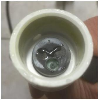
After proper cleaning, water adhesion was 100%.
