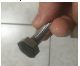
Cleaning tool can be a bolt with a flat surface on top, doubled sided tape and wet & dry sandpaper 300 to 600 grit. Another possibility is a length of dowel or broom handle, cut squarely with the doubled sided tape and wet & dry sandpaper. Diameter needs to be 20 to 25mm diameter to cover the whole area of the probe face. Always use water to wash away any material taken off the probe surface.
